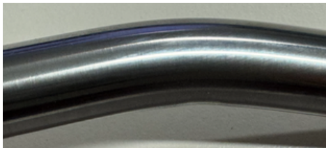
Bend test - No detachment, ensuring strong adhesion
